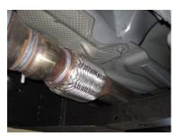
2. To remove stock exhaust, unclamp it at the ball flange behind the Y-pipe. Make sure to leave all rubber grommets in the factory location. **You will re-use stock clamp.** For easier removal of exhaust, cut behind the muffler. Use WD-40 to remove hangers from grommets.
