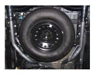
7. Install passenger side tailpipe #C into muffler at least 1.5" to 2". Use clamp #G to secure pipe to muffler. Do not tighten. The tailpipes will both lean towards the driver side for clearance. Insert welded hangers into rubber grommets.
