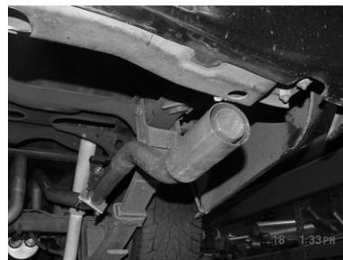
INSTALL EXIT PIPES # F ONTO OVERAXLE TAILPIPES USING CLAMP # J. ADJUST FOR YOUR PREFERENCE. NEXT ROTATE PIPES FOR BEST CLEARANCE AND ALIGN TO FRAME RAIL. TIGHTEN ALL CLAMPS AND BOLTS STARTING FROM THE HEADPIPE AND WORK BACK. INSTALL STAINLESS STEEL TIPS.
