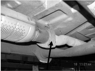
UNBOLT STOCK HEADPIPE AT THE 3 BOLT FLANGE DIRECTLY BEHIND THE CATALYTIC CONVERTER. CUT STOCK TAILPIPE OFF RIGHT BEHIND THE STOCK MUFFLER. LEAVE ALL FACTORY RUBBER GROMMETS IN PLACE. SPRAY WD-40 ON ALL RUBBER GROMMETS FOR EASY REMOVAL.
