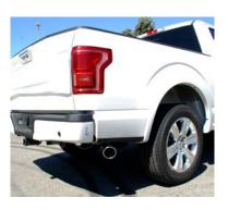
MAKE SURE YOU HAVE A 1" CLEARANCE ON ALL RUBBER BRAKE LINES, SHOCK BOOTS, TIRES, FUEL LINES, ETC..
