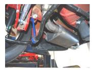
3. Now install the passenger side muffler assembly #B by sliding the metal hangers into the rubber grommets. Then do the same for the driver side muffler assembly #A.
