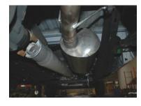
4. Install muffler #B onto headpipe  $1\frac{1}{2}$ "-2" with the louvers facing towards the converter. Muffler outlet will be at the 9 o'clock position. Use a jack stand to support the
