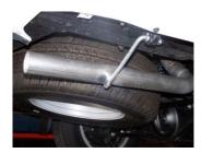
7. Install the exit pipe #D onto the tailpipe. Secure together with clamp #F. Do not tighten. Roll the exit pipe until it is at the correct angle for your vehicle. Insert welded hanger into rubber grommet.
