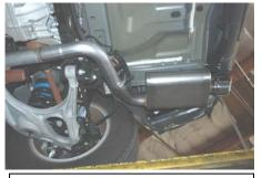
3. Install the driver side muffler assembly onto the factory pipe. and into the factory rubber grommets. Do not tighten.
