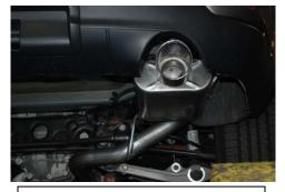
5. With the muffler assembly in place align the tip so it is centered in the exhaust outlet. You may need to use something like a rag to hold the tips in place while the clamp is being tightened.
