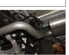
5. Install the Passenger side muffler assembly onto the factory pipe and into the factory rubber grommets. Do not tighten.
