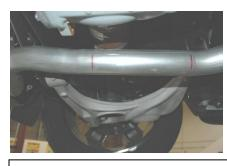
2. To remove the driver side exhaust measure 8" from the bend located under the rear end forward. Mark and cut with a hack saw or cut off wheel. Leave the factory rubber grommets in place they will be re used.
