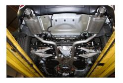
6. With both mufflers in place align both parts so they match each other and are centered in the exhaust outlets. You may need to use something like a rag to hold the tips in place while the clamps are being tightened.
