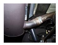
2. To remove the stock exhaust, unbolt band clamp located just behind your factory muffler.
