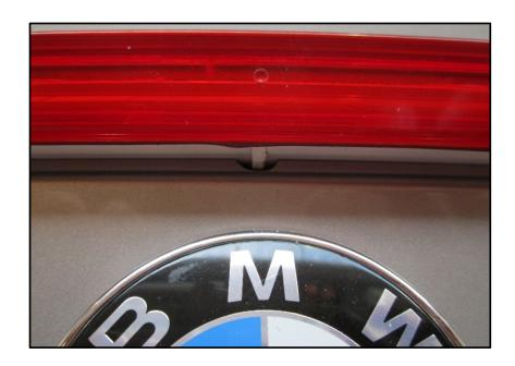
8. Ensure that the 3<sup>rd</sup> brake lamp is centered after installation.
