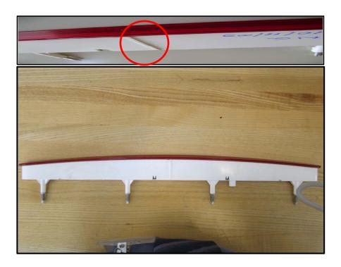
3. The new brake lamp may have a guide as indicated in the picture. If the lamp has a guide, proceed to the next step. If the lamp does not have a guide, finish the replacement.
