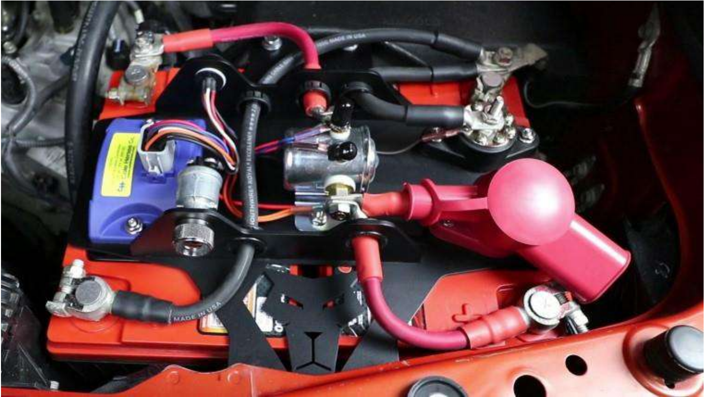
Final installation. Ensure all post clamps are tight.
