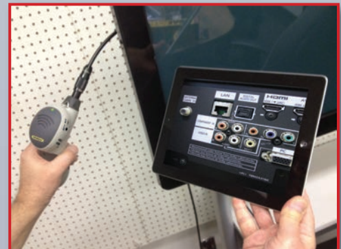
iBorescope makes it easy to identify the jacks on the back of rack or wall-mounted equipment
