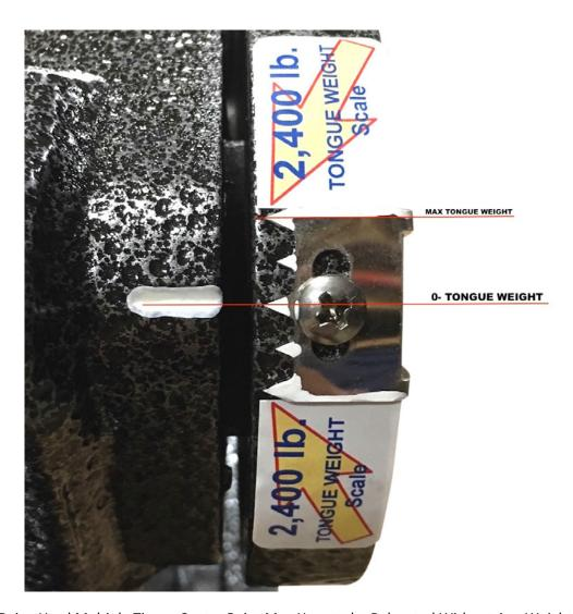
After Being Used Multiple Times, Center Point May Have to be Relocated Without Any Weight on Hitch (Simply unscrew set screw & relocate to center & retighten).
