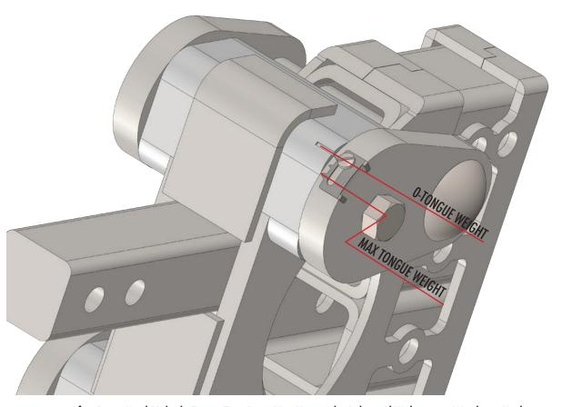
After Being Used Multiple Times, Zero Point May Have to be Relocated Without Any Weight on Hitch (Simply unscrew set screw & relocate to zero point & retighten).
