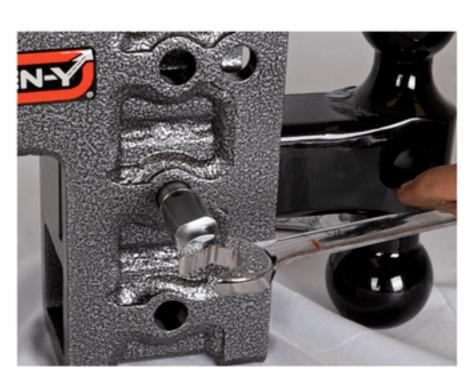
3. Pull the sleeve out & remove pin.
