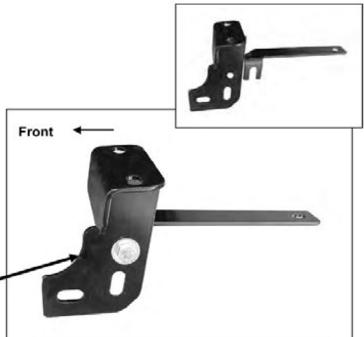
(Fig 4A) Driver side Support Bracket in "no tow hook-with bumper support" position
