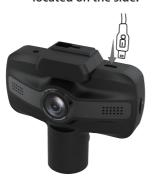
④Run the power cable around the vehicle's trim and insert the car charger into the vehicle's cigarette lighter port as shown.
