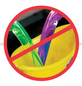
Topping off the system with a non-compatible coolant may reduce the original inhibitor levels and corrosion protection.
