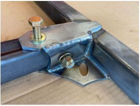
6. Test Fit Jet Ski before use and adjust bunks to fit best using either of the three mounting holes on the Side Wings. Each gusset has a hole for ratchet straps. Double check all hardware and tightness of straps before each use.
