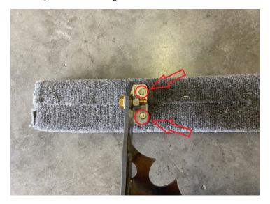
5. Bolt Hitch Tube to Main Frame using the 2 supplied 1/2-20x4" GR8 Bolts (2 washers and one nylock per bolt). Make sure to tighten bolts to at least 75 ft lbs before using.
