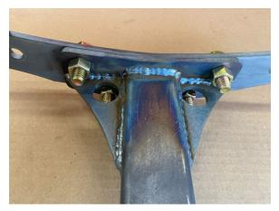
2. Bolt "Bunk Mounts" on using 4x (1/2-20x1" GR8 Bolts) with two washers and one nylock per bolt. Bolt on from outside of Side Wings as shown below.
