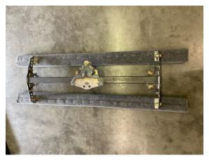
4. With bunk mounts in place and centered, drill pilot holes in the bunks using your 3/32 Drill Bit in the two holes of the metal bracket and screw in the provided 1/4 lag bolts. DON'T OVERTIGHTEN AS YOU MAY STRIP OUT THE WOOD (It may be easier to do this step one mount at a time so the wood doesn't shift on you when moving to the next mount.
