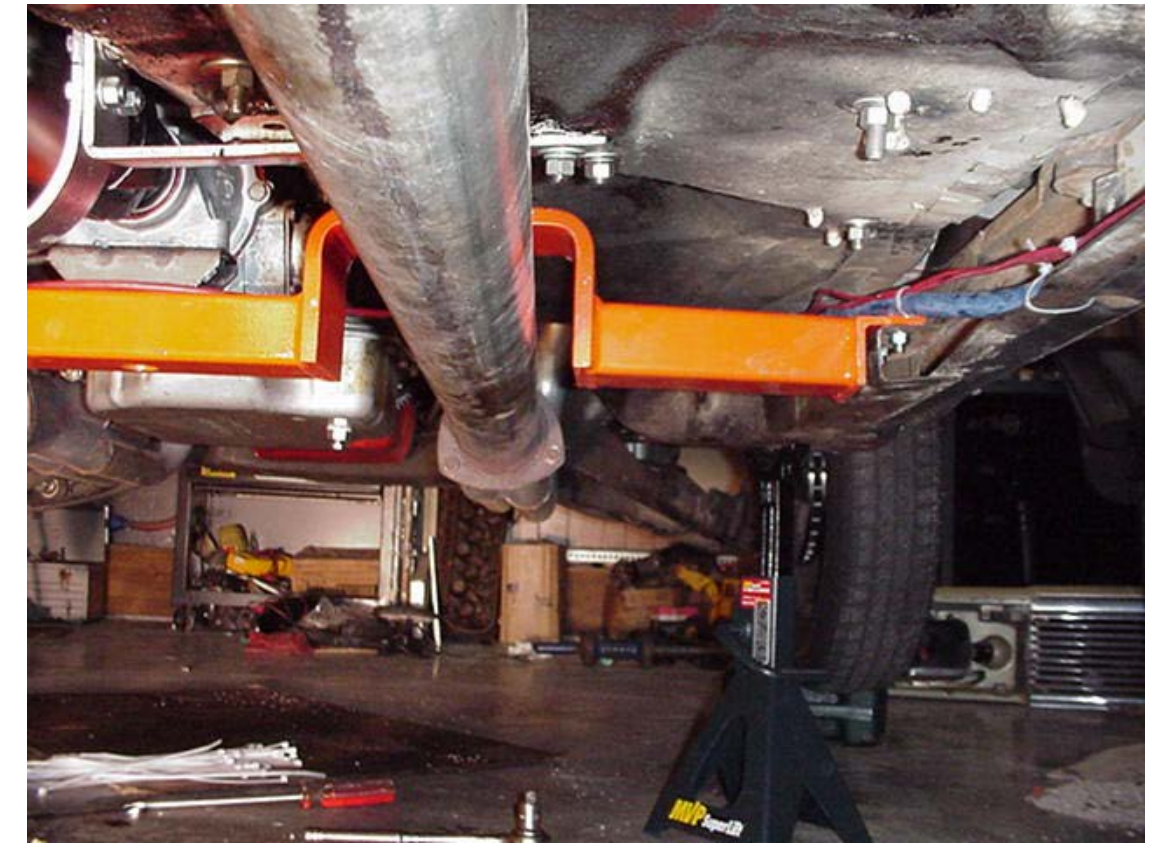
Same for the passenger side. There's plenty of room for a bigger pipe.
