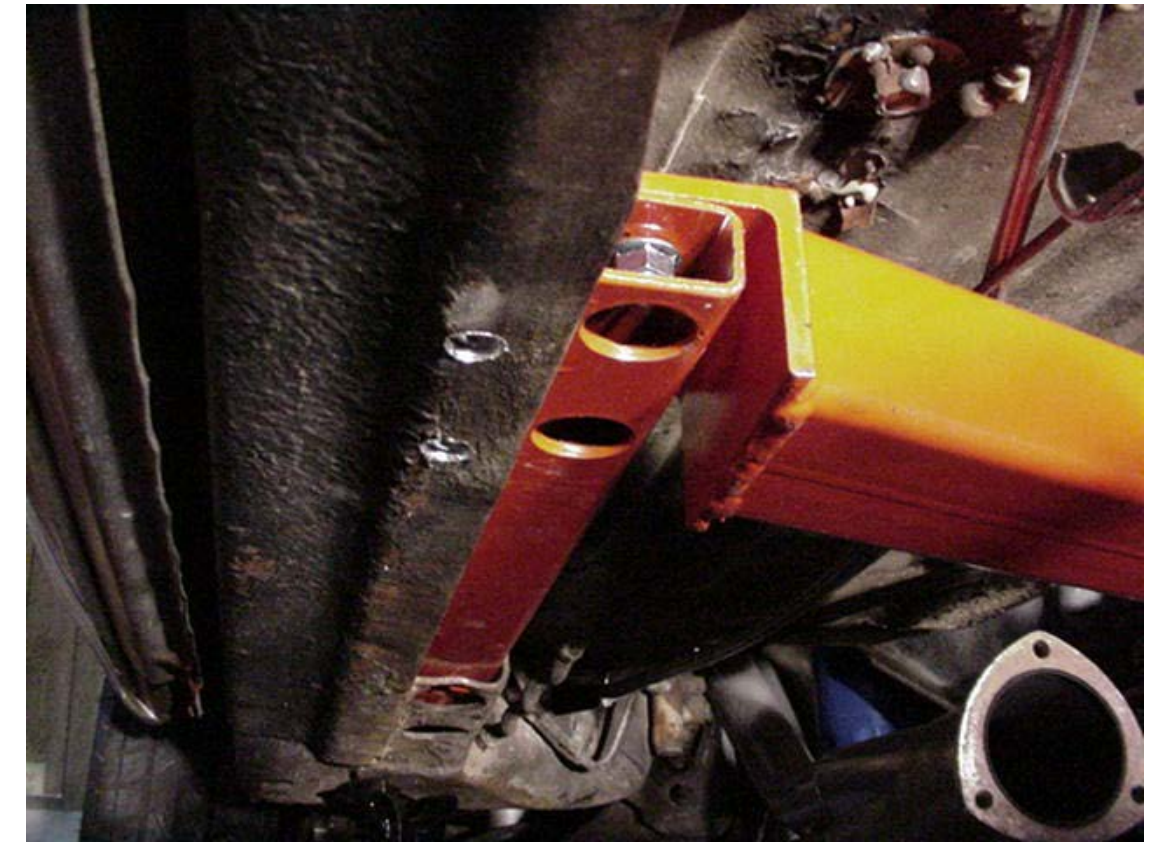
Here is where I used the supplied template to drill the two holes into the frame to securely mount the rear part of the extension. This was the hardest part, but drilling two holes isn't too difficult!
