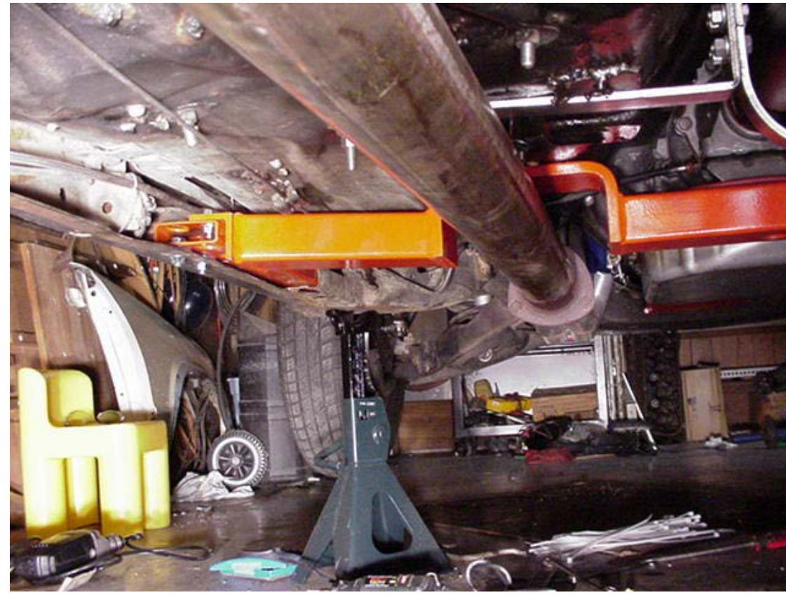
Here's the driver side exhaust pipe. It is a 3" pipe, and has PLENTY of room!
