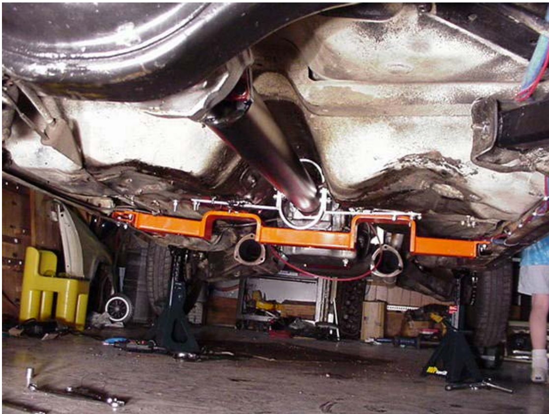
Next step is to re-install the driveshaft. Note that it is a 3.5" diameter shaft and it is TIGHT around the driveshaft safety loop.
