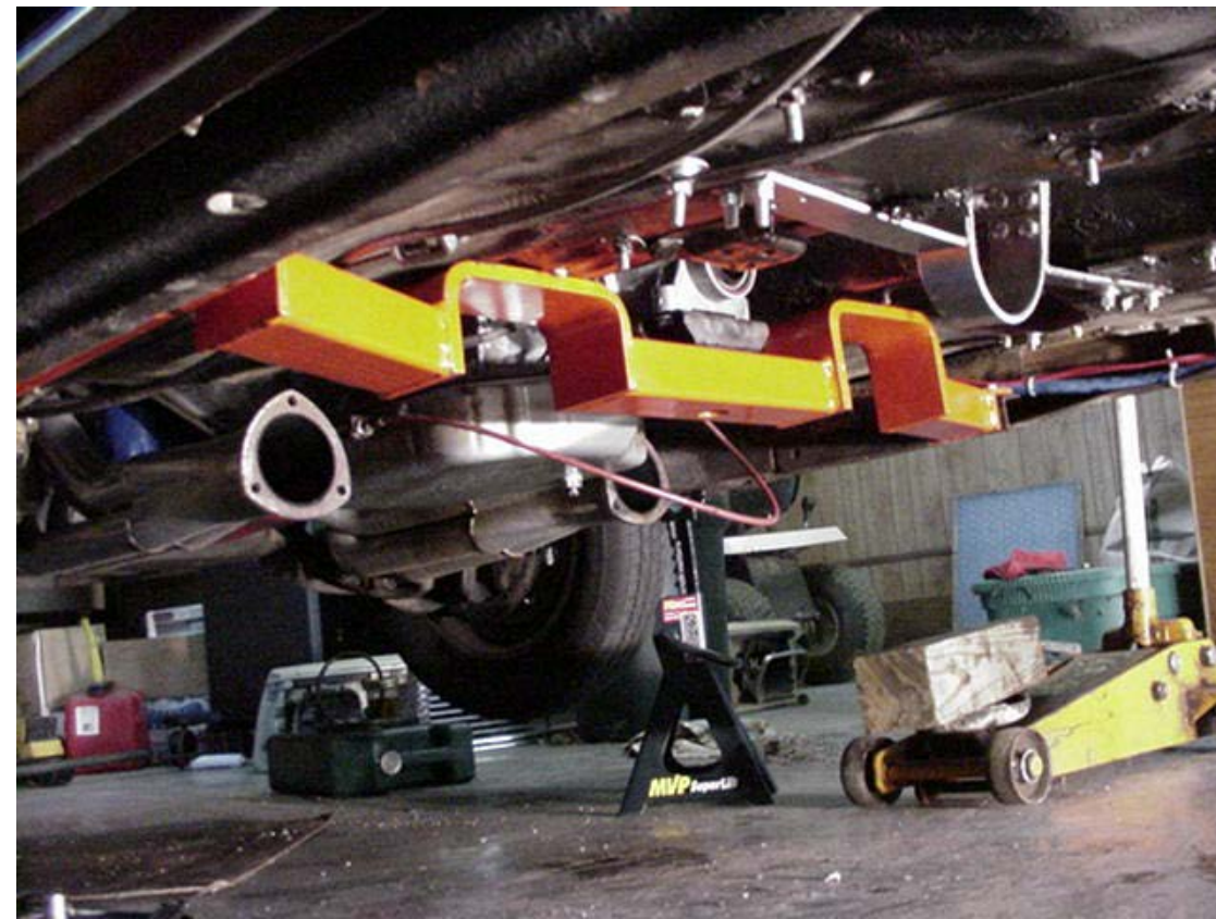
OK, everything is lined up and tightened down. I removed the floor jack, and the transmission is resting on the crossmember.
