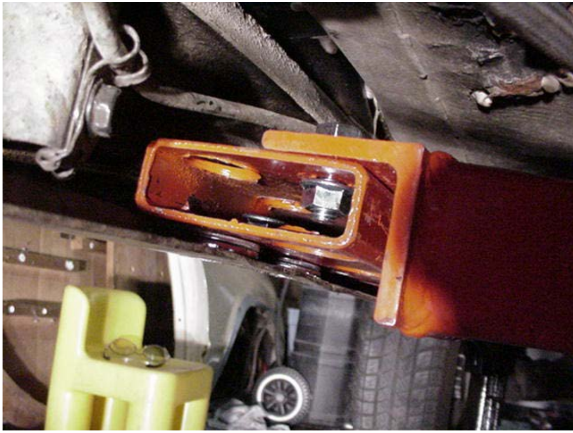
Since the framerail has a slight drop on the inside, you have to use some shims that come with the kit between the extension and framerail where the bolts pass through.
