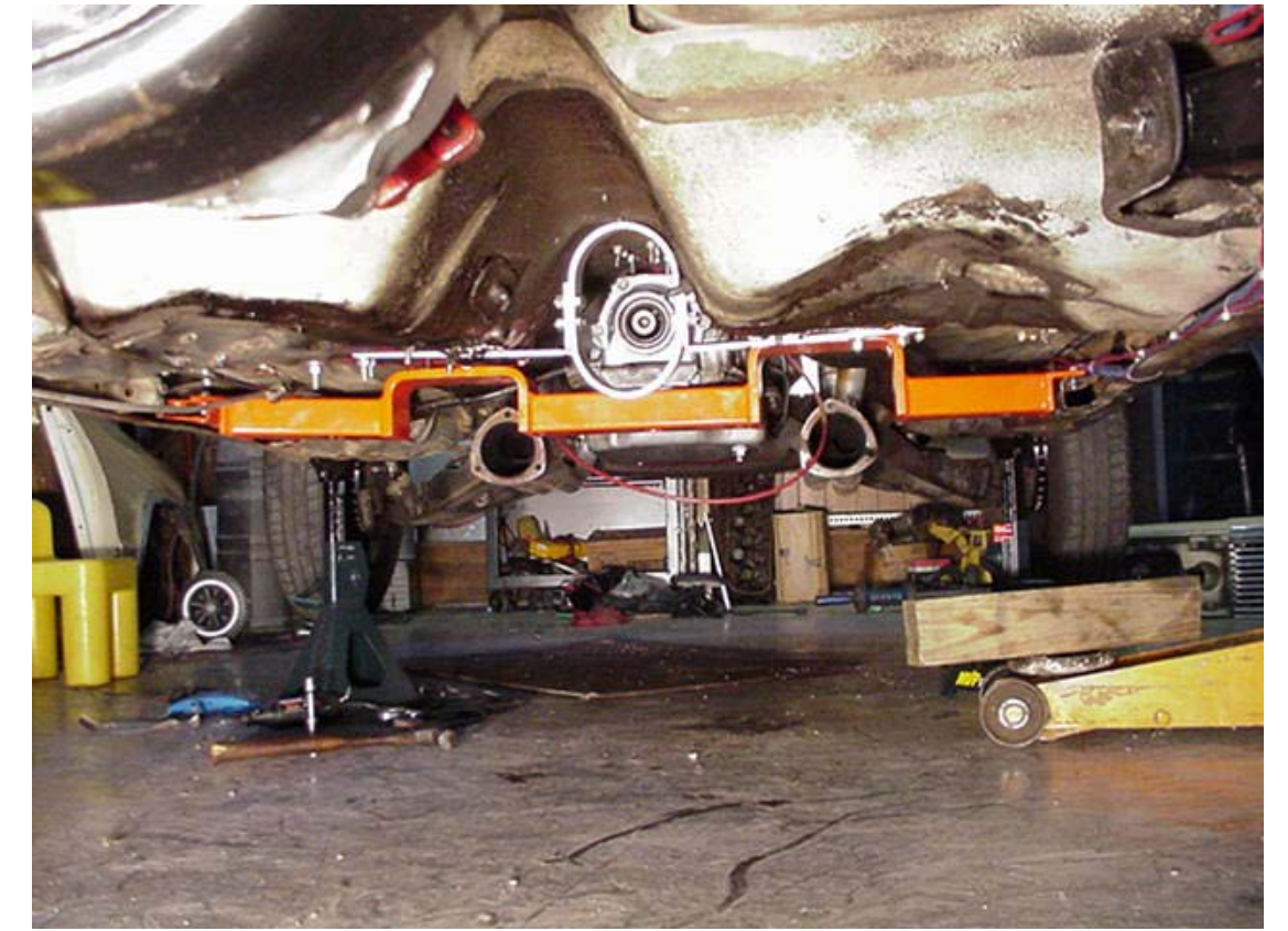
Here's the rear view of the crossmember after it has been bolted into place. Note that my shifter cable is hanging down. I had to re-route it to where it rests on top of the crossmember on each side of the transmission mount area.
