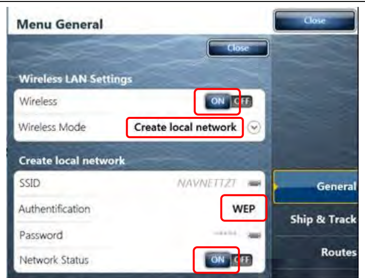
Wireless: ON (TZT9/14/BB only) Wireless Mode: Create local network Authentication: WEP (TZT9/14/BB only) Network Status / Local Network: ON
