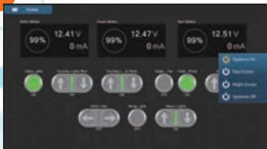
Digital Switching on Your Fingertips Monitoring and Controlling digital switching CZone system from your NavNet TZtouch2.
