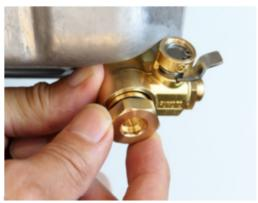
The versatility of the SX-series valve allows installation without an adapter on some cars and trucks that may have previously required one.
