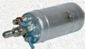
Bosch High Output Pump 200 liters per hour (52.5 gph) at 72 psi (5 bar) at 13A, filter optional Part No. FP044
