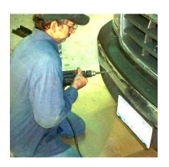
Step 3: Align grille guard to truck and mark holes. Drill 1/2 inch holes (2 per side) through chrome bumper and bumper support bracket (installed in step 2).
