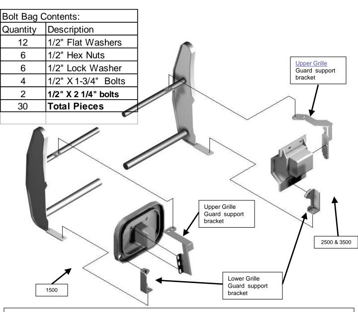
**Step 1:** Raise the Hood. Remove the two nuts on the side of the frame behind the frame cap (2500, 3500). Remove the two or three nuts on the back of the frame cap (1500). Insert upper grille guard support bracket and align to the two bolts, replace nuts and tighten. (Hint: the bracket should be below the hood 3/8" when the hood is closed).
