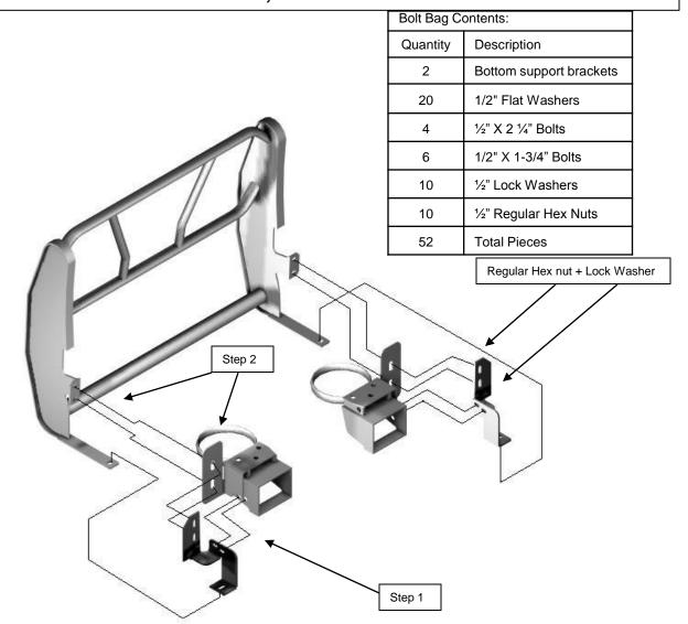
**Step 1:** Install bottom support bracket behind frame horn. NOTE: You must use regular ½" hex nuts and ½" lock washers on the bolts going through the truck frame!! You will access the bolt head through a small hole located on the inside/bottom of truck frame when you are tightening.
