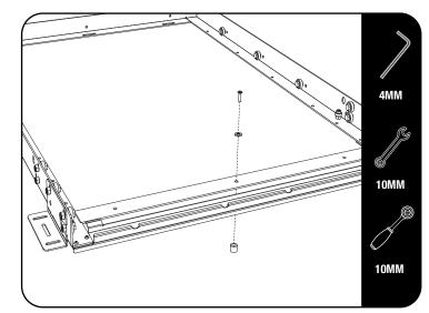
Place the frame back onto the load bed and secure using the fasteners and spacers supplied. The spacers (Item 5) are to be used when the mounting points are in a "dip" and not on a raised section by placing it over the rivnut so that the frame rests on the spacer.
