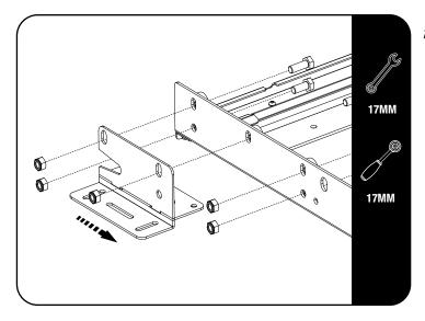
Position the frame, front to back and left to right. Load beds vary with each manufacturer, so the exact positioning of the frame will vary from vehicle to vehicle. I t is advisable to get all mounting points in the center of the raised sections that run the length of the load bed, however in the event of mounting points not lining up with raised sections, spacers have been provided.
