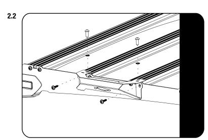
Secure the Handle Light Rack Bracket (Item 1) to your Roof Rack using M8x12 Button Heads, M8 Schnorr Washers, M8 Half Nuts & M6 x 25 Self forming Screws (Items 2,3 & 4).
