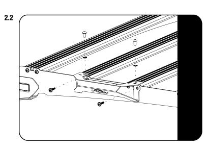
Secure the Handle Light Rack Bracket (Item 1) to your Roof Rack using M8x12 Button Heads, M8 Schnorr Washers, M8 Half Nuts & M6 x 25 Self forming Screws (Items 2,3 & 4).
