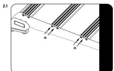
Slide two M8 Half nuts (Item 4) into the T-Slot and Remove the Self forming Screws indicated.
