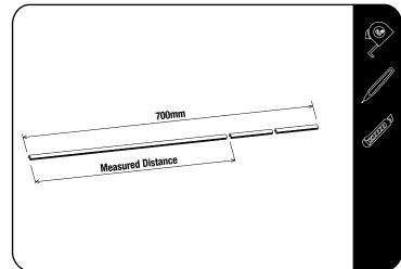
Using the measurement from 2.4, cut the T-Slot Rubber (Item 17), removing 20mm extra to allow for the bolts to pass through. Cut the remaining piece into 2 as shown.
