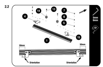
Assemble a RH Release Bracket (Item 4) and a LH Release Bracket (Item 15) with two Quick Release Bobbins (Item 14) to each Slat (Item 1) using the Thin Nuts inserted in 2.1, four M8 Flat Washers, four M8 Spring Washers, four M8x16 Button Head Screws and four M8x30 Cap Screws (Item 5, 6, 7 & 13)
