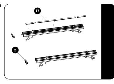
Insert the T-Slot Rubbers into the T-slot of each Slat with the M8x35 Hex Head Bolts (Item 16) positioned as shown.
