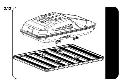
Lower the Cargo Box onto the rack making sure the Quick Release Feet align with the rack mounted Catch Brackets.
