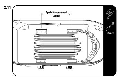
Apply the measurement from 2.10 to center the Narrow Box Brackets and fully tighten. Finish off by placing M8 Nut Caps (Item 12) on the M8 Nyloc Nuts.
