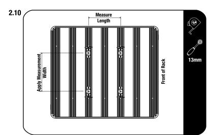
Apply the measurement from 2.4 to the centers of the Catch Brackets and fully tighten the Catch Brackets. Finish off by placing M8 Nut Caps (Item 12) on the M8 Nyloc Nuts.
