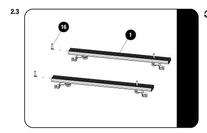
Turn the assembled slat over and slide four M8x35 Hex Head Bolts (Item 16) into the assembled slats as shown.
