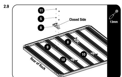
Taking into account the length and width of your cargo box, choose where you'd like to position it on the rack. This will determine where you need to fit the Catch Brackets (Item 8 & 10).
