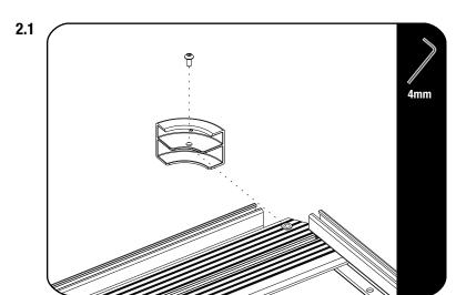
Determine where on the Side Profile you would like to mount your antenna. Remove the corner closest to that position.
