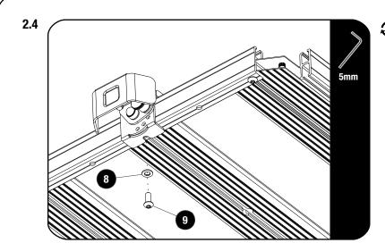
Align the bottom slot in the Antenna Mount with the bottom hole in the Side Profile.
