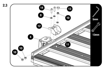
Slide two M8 Nyloc Nuts (Item 10) into the Side Profile.
