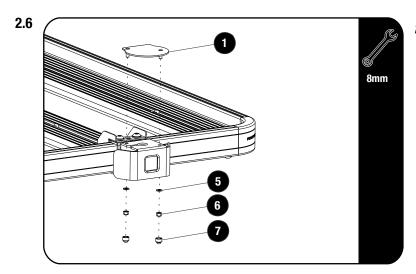
To mount an antenna with a magnetic base, secure the Antenna Mount Plate (Item 1) to the already secured Antenna Mount using two M5 Flat Washers and two M5 Nyloc Nuts (Item 5&6). Finish off by placing two M5 Nut Caps (Item 7) on the M5 Nyloc Nuts.
