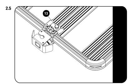
Fully tighten all the bolts and refit the corner. Finish off by placing a M8 Nut Cap (Item 13) on the M8 Nyloc Nut.
