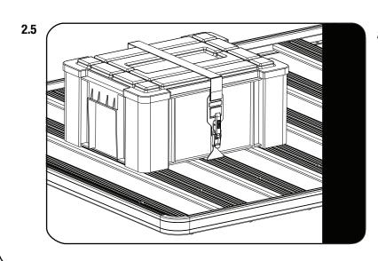
With the latch in the open position and secured onto the catch mount, adjust the strap to the correct length to fit the storage box.
