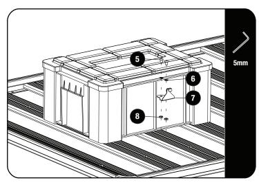
Slide two M8 Half Nuts (Item 8) into the T-Slot in the slat on the opposite side of the storage box. Using two M8 Schnorr Washers and two M8 x 12 Button Head Bolts (Item 6 & 5) secure the Lock Catch Mount (Item 7) so that it will sit under the storage box.
