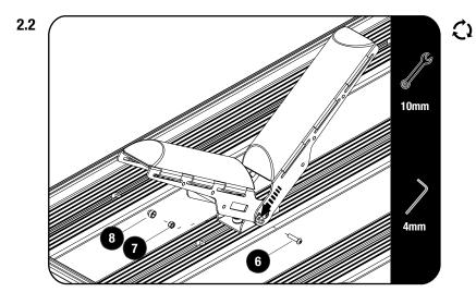
Each Carrier has five settings, allowing you to adjust the angle. (Refer to Step 2.3).
