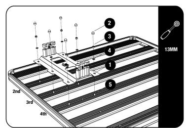
Slide 2 M8x16 hex bolts (item 5) into each of the 2nd, 3rd and 4th slats t-slot. Place the Rotopax mounting plate (item 1) over the bolts. Move the mounting plate into the desired position by using the Rotopax tank before securing it with items 3 and 4. Finnish it of by placing a M8 nut cap (item 2) over each of the 6 nyloc nuts (item 3).
