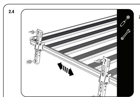
Set final position with a MaxTrax mounted onto the brackets and fully tighten brackets.
