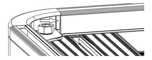
( **B** ) Place one End Piece and the Joiner Pieces (Items 2, 5) onto either side of the Rack, making sure that the "Feet" of the End and Joiner Pieces sit inside the U-channel as shown. Line up the mounting holes in the End and Joiner Pieces with the Nyloc Nuts inserted in Step 2A and loosely secure them to the Rack using the M8 x 25 Button Head Bolts (Item 1) supplied.
