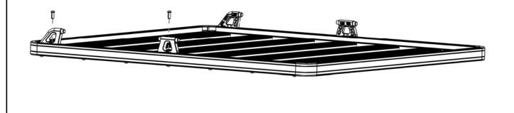
( C ) Fit the Pipes (Item 4) between the End Pieces and Joiners. Loosely fit and secure the remaining End Pieces. Center the Side Rail assemblies left to right and tighten all bolts.
