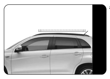
With the help of a friend, hold your Front Runner Roof Rack over your vehicle's Flush Rails. Find the best position to mount.
