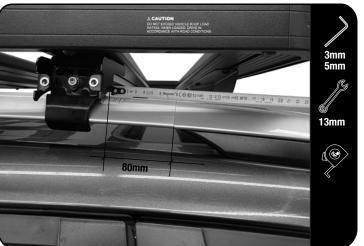
Place your Tray on the vehicle positioning all the feet so that they rest on top of the roof rails.
