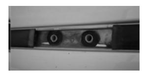
(**D**) Clean the area around the threaded holes in the vehicle's roof using a rag and some methylated spirits / denatured alcohol. Place some silicone around each threaded hole in the vehicle's roof and the two cut-outs in each of the Spacers (Item 11) as shown. Position the Spacers into the vehicle's gutters, lining up the cut-outs in the Spacers with the threaded holes in the vehicle roof.
