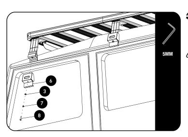
Tightening Torque 16Nm / 11.8 ft lbs
