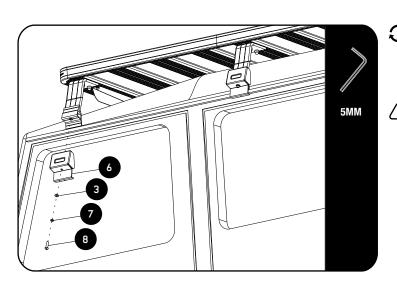
Secure the Gutter Clamps (Item 6) using M8 x 30 Button Heads, M8 Spring Washers and M8 x 16 x 1.6 Flat Washers (Items 3, 7 & 8). Check that the Clamp is seated correctly under the gutter before tightening.
