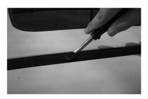
(C) Loosely join the Front and Rear Foot Rails together using the M6 x 16 Button Head Bolts, M6 Flat Washers, M6 Nyloc Nuts and Joiner Plates (Items 7, 8, 9, 10).
