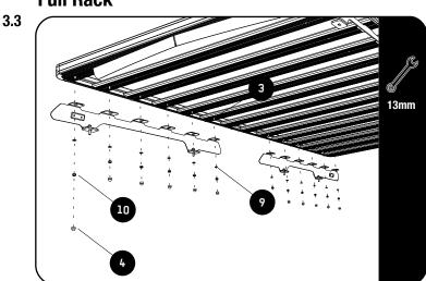
Fit your Roof Rack to the Foot Rails using M8 x 20 Hex Bolts, M8 x 16 x 1.6SS Flat Washers and M8 Nyloc Nuts (Items 3, 9 & 10).
