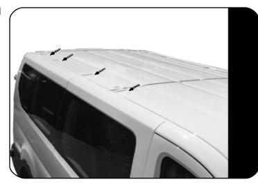
$\bigcirc$  0n the roof, remove the hole plugs shown in 2.1.
