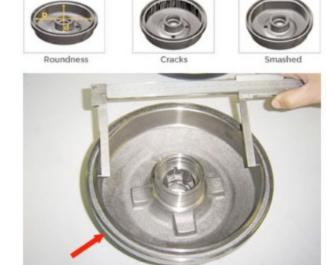
TIP: never assembly new linings or brake shoes on uneven braking surface, this will cause brake inefficiency. If the inner diameter of the drum is less than the maximum allowed diameter, it can be machined by a service technician. If not, it must be replaced.
