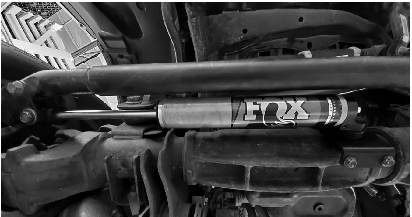
Figure 9: Reasonable shaft clearance
