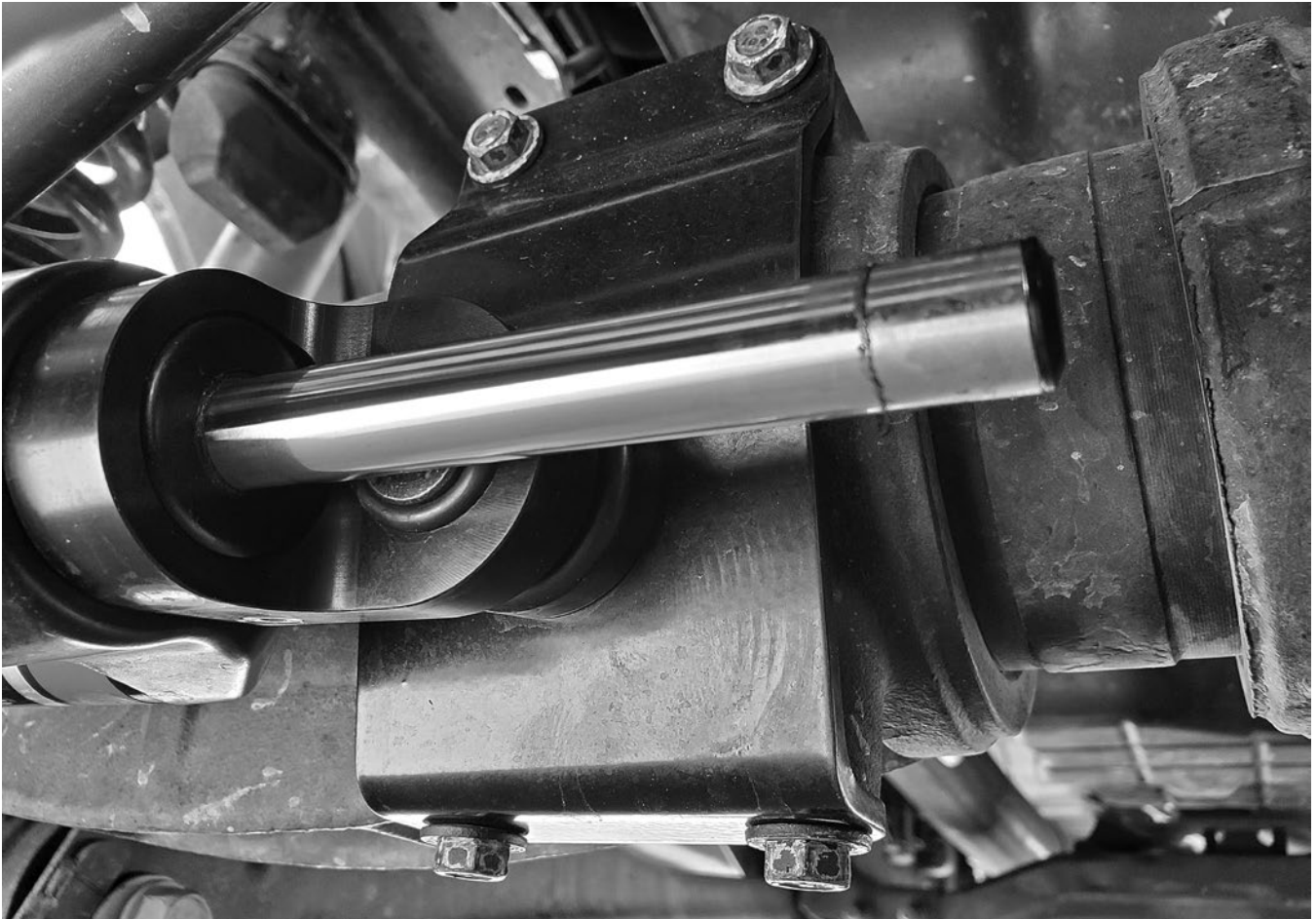
Figure 6: Axle bracket installed
