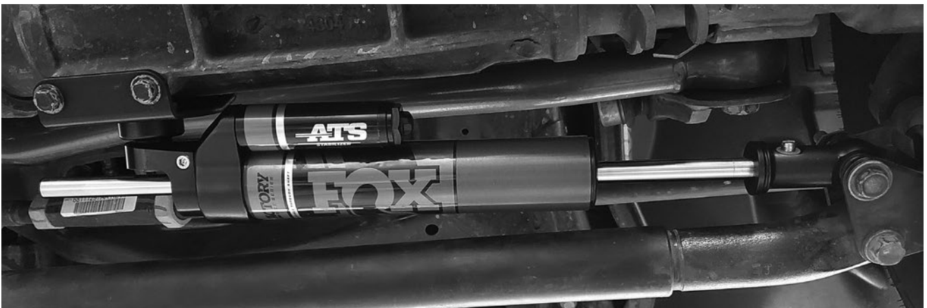
Figure 7: Correct stabilizer installation with wheels pointed straight, ATS shown.
