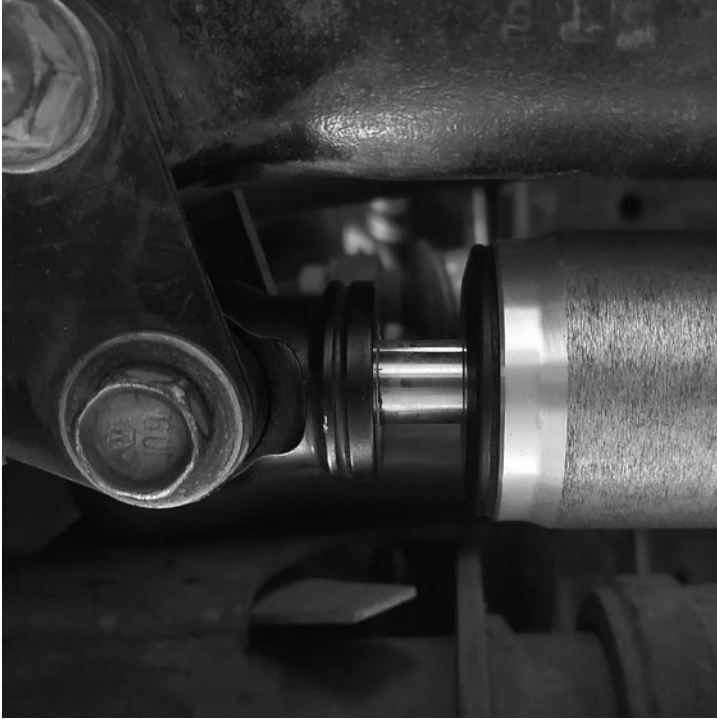
Figure 8: Reasonable shaft clearance
