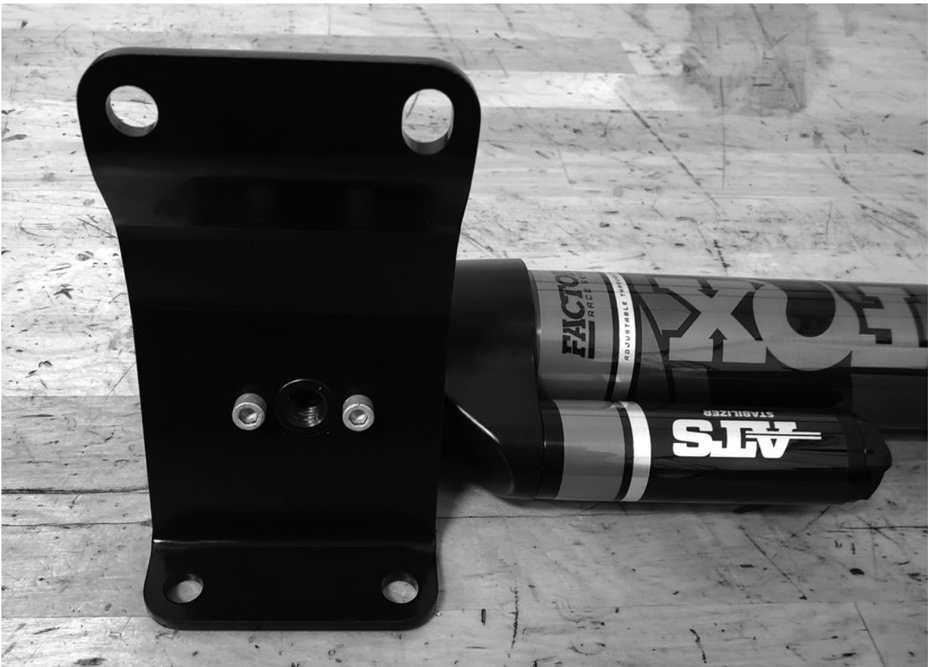
Figure 5: Replacement bracket attached
