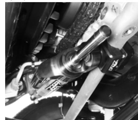
Fig. 2: Stabilizer clamped to drag link
