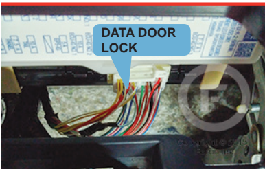
⑥ Under fuse box
