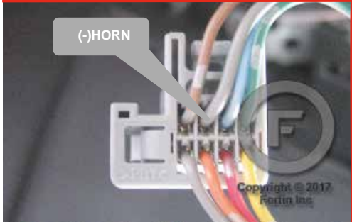
⑦ At steering column * Test wire before connecting
