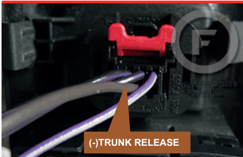
④ BCM, left of the steering column
