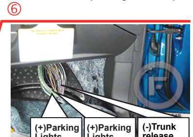
Harness under passenger-side carpet.
