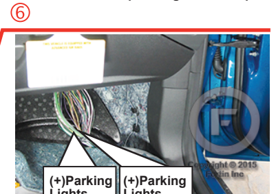
Harness under passenger-side carpet.
