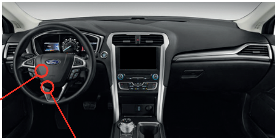
① Gateway module, Behind OBD-II connector
