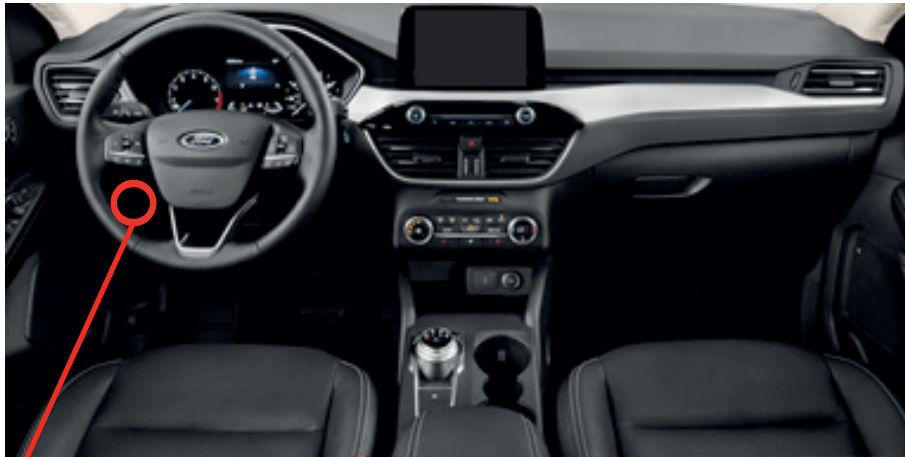
① Gateway module, Behind OBD-II connector
