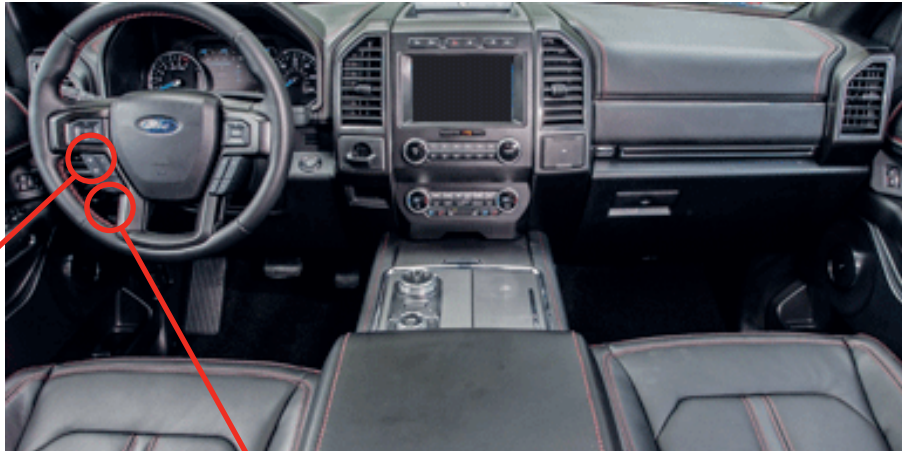
① Gateway module, Behind OBD-II connector
