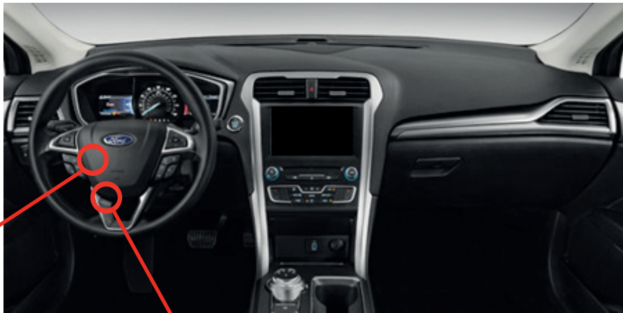
① Gateway module, Behind OBD-II connector
