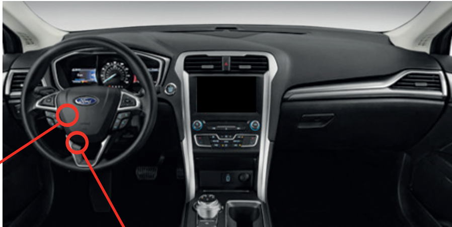
① Gateway module, Behind OBD-II connector
