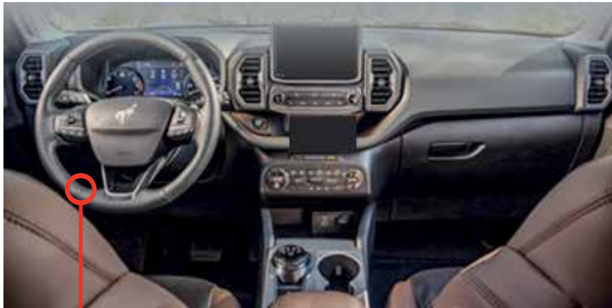
① Gateway module, Behind OBD-II connector
