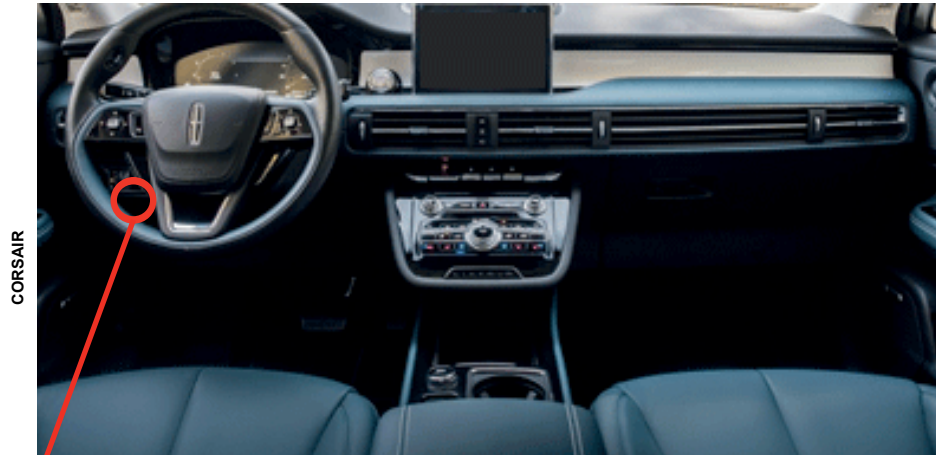
① Gateway module, Behind OBD-II connector
