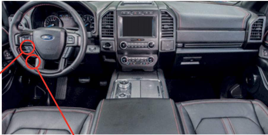
① Gateway module, Behind OBD-II connector
