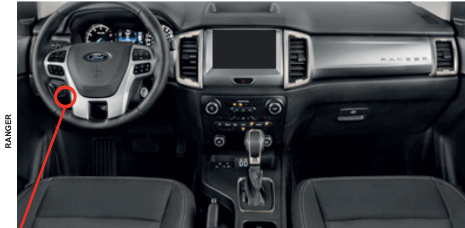
① Gateway module, Behind OBD-II connector
