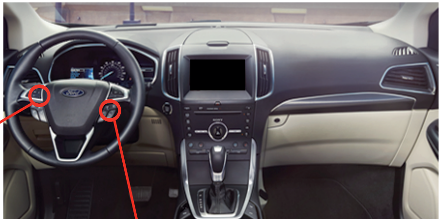
① Gateway module, located at dash board driver's side,
