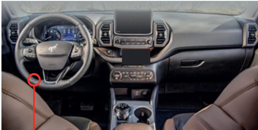
① Gateway module, Behind OBD-II connector
