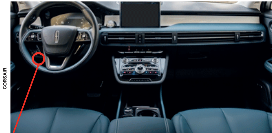
① Gateway module, Behind OBD-II connector
