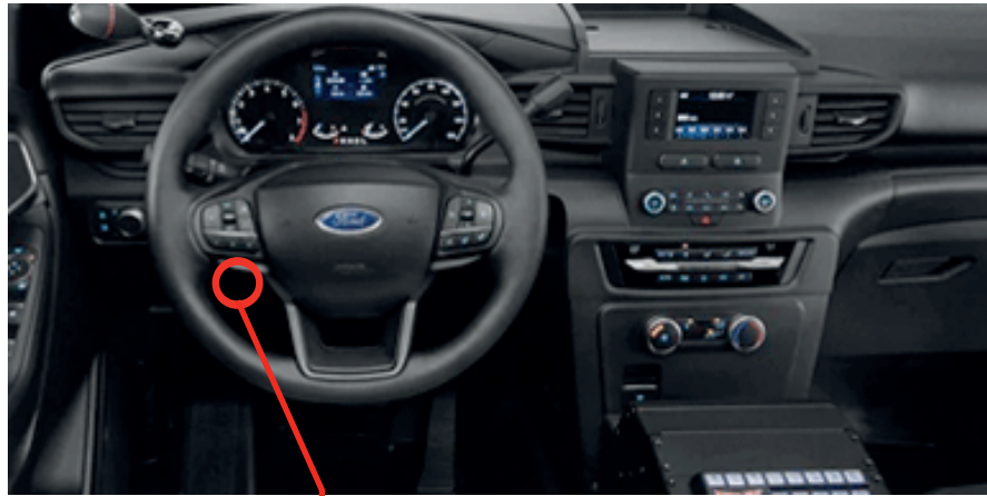
① Gateway module, Behind OBD-II connector - located behind driver side fusebox
