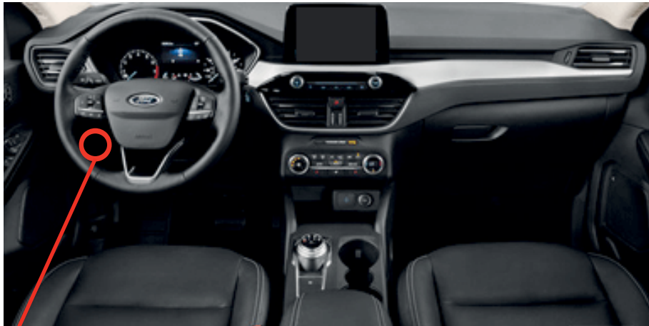
① Gateway module, Behind OBD-II connector
