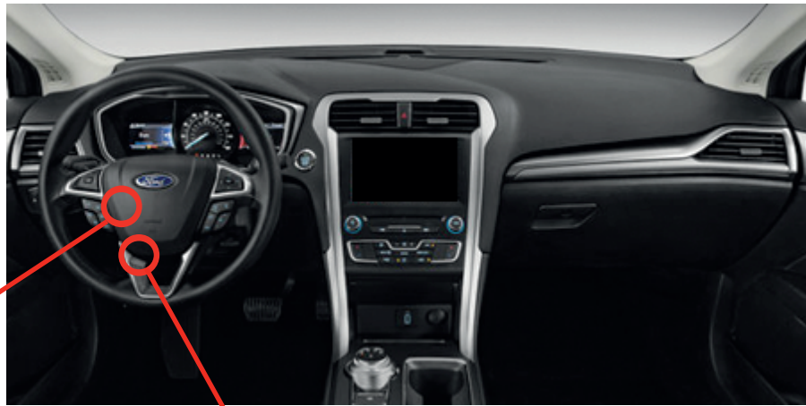
① Gateway module, Behind OBD-II connector
