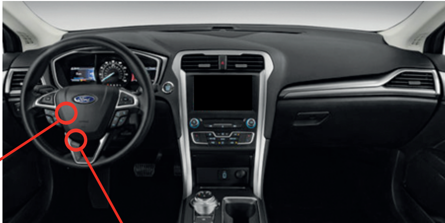
① Gateway module, Behind OBD-II connector
