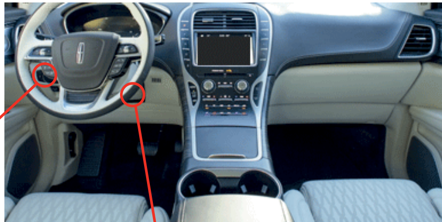
① Gateway module, Behind OBD-II connector
