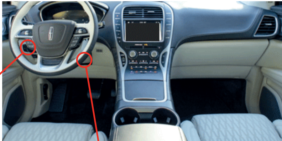
① Gateway module, Behind OBD-II connector II
