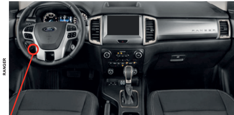
① Gateway module, Behind OBD-II connector
