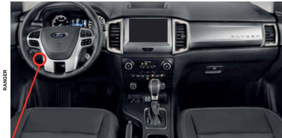
① Gateway module, Behind OBD-II connector
